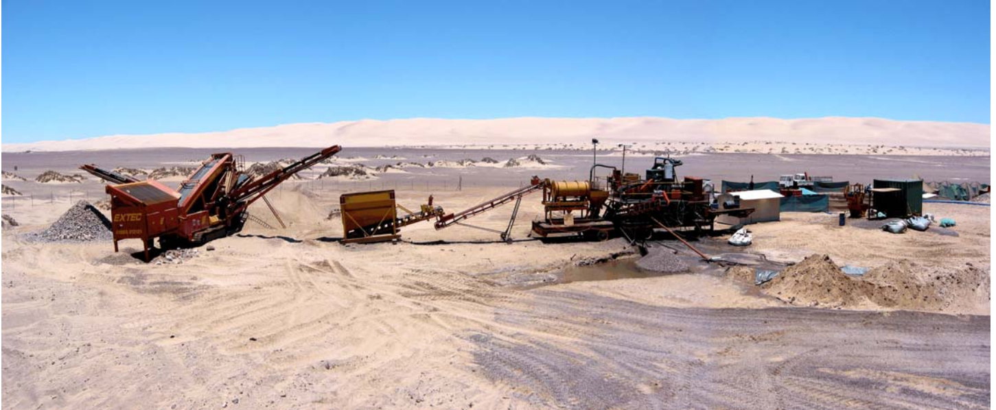
Figure 3. Photograph of the processing facility at the Skeleton Coast Diamond Project incorporating Screening unit and DMS Plant.
